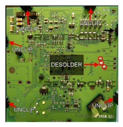
Remove the PCB and locate the brown component. Remove this component and reassemble the board.
