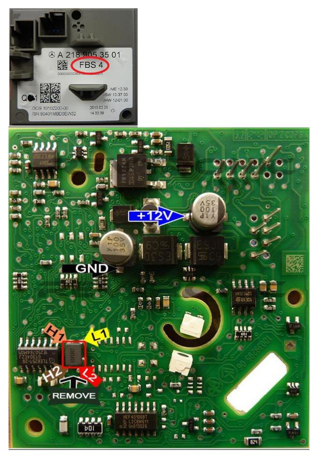
SLS W197 – EZS CONNECTIONS – JUMPER 2 – ON
